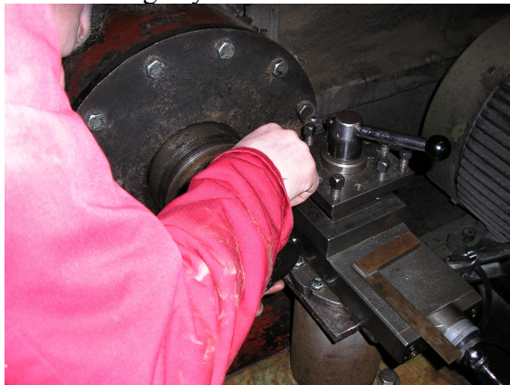
Left: FirScot engineers machining the shaft
